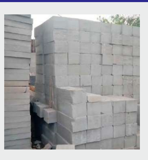
Built with Aerocon Blocks (50% less weight than generic bricks)
